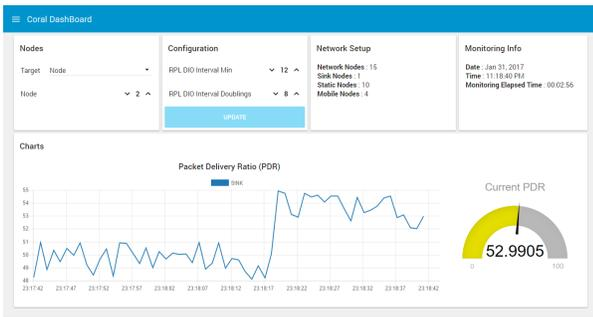
Fig. 2. The CORAL dashboard shows the impact of the dynamic RPL configuration in real-time
